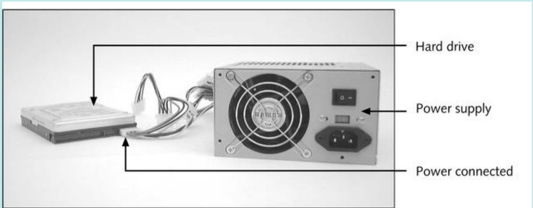
Figure 1-21 A hard drive receives power from the power supply by way of a power cord connected to the drive
