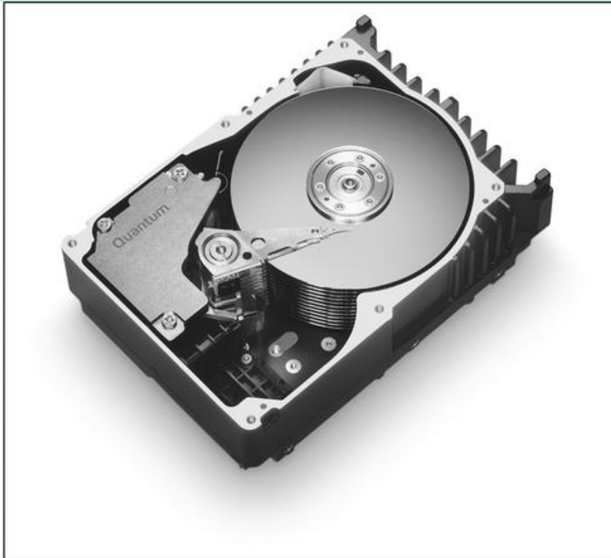
Figure 1-17 Hard drive with sealed cover removed
