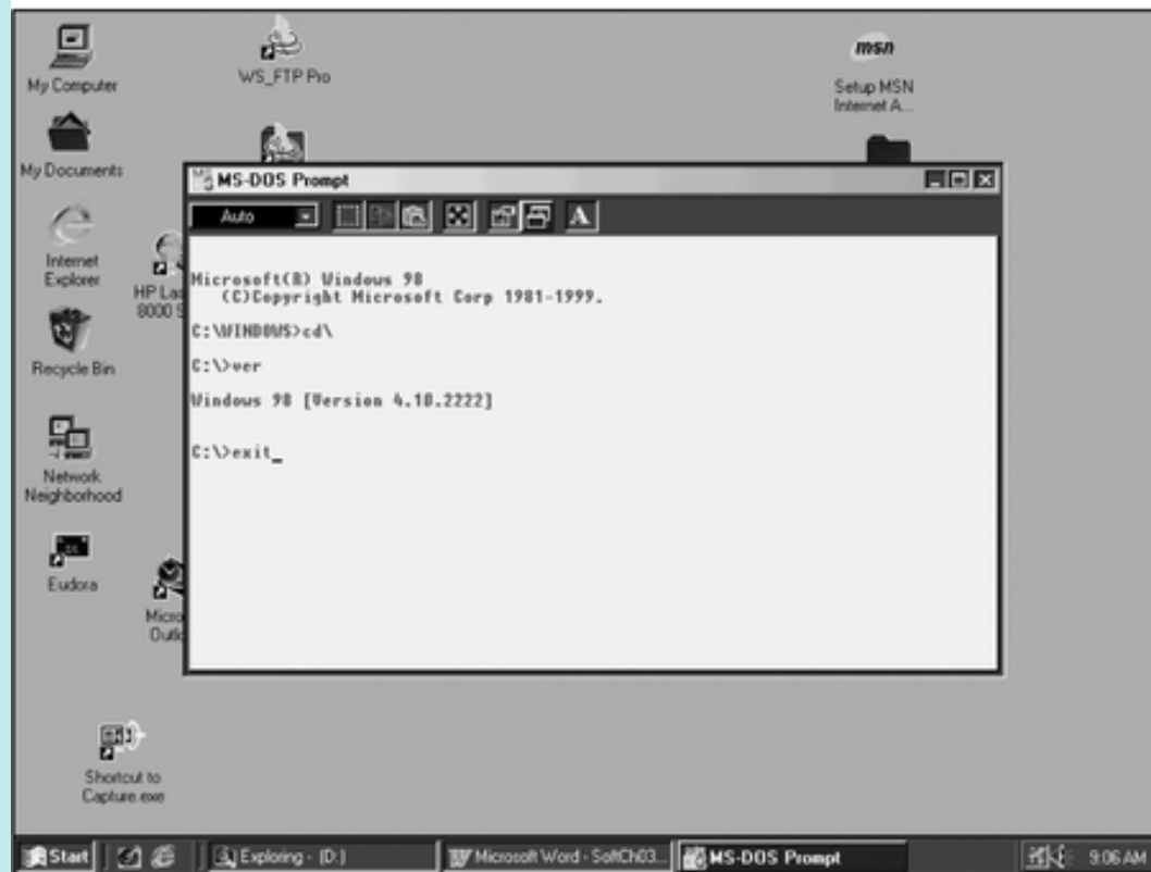
Figure 3-11 An MS-DOS Prompt window operates in the virtual real mode provided by Windows 9x
