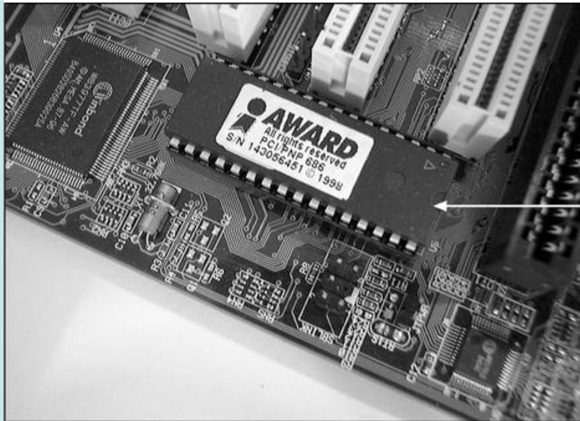
Figure 6-1 The ROM BIOS on newer motherboards can be upgraded using software provided by the BIOS manufacturer
