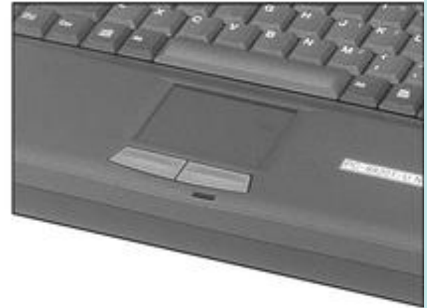
Figure 10-23 The most common pointing devices: a mouse, a trackball, and a touchpad
