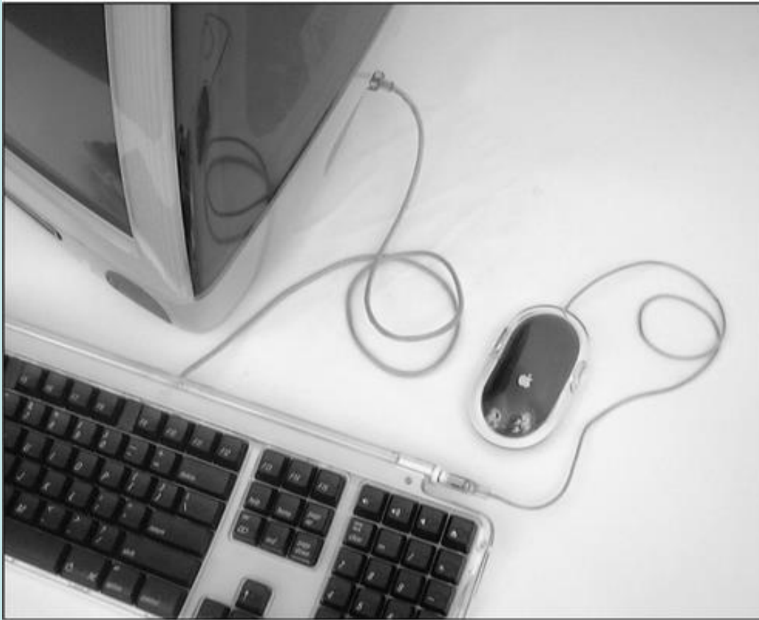
Figure 10-11 A keyboard and a mouse using a USB port daisy-chained together
